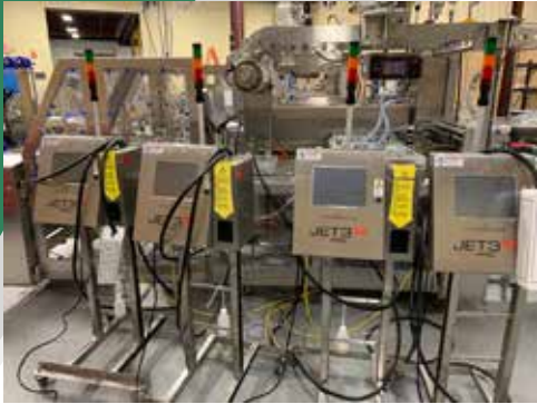
4 Head CIJ Printer needs 4 Controllers
