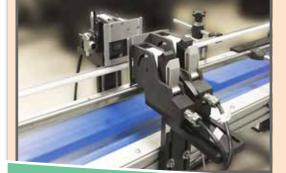
Can be set up to print on both sides of a box at the same time
