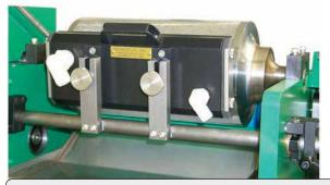
Enclosed Doctor Blade design allows for highspeed operations and minimal ink waste.
